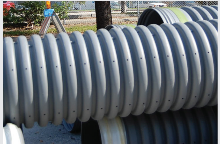
Remarkably, an FDOT spec change was needed to explicitly prohibit drilled corrugations, as shown in this photo of polypropylene pipe in the City of Miami Beach, 2011.
