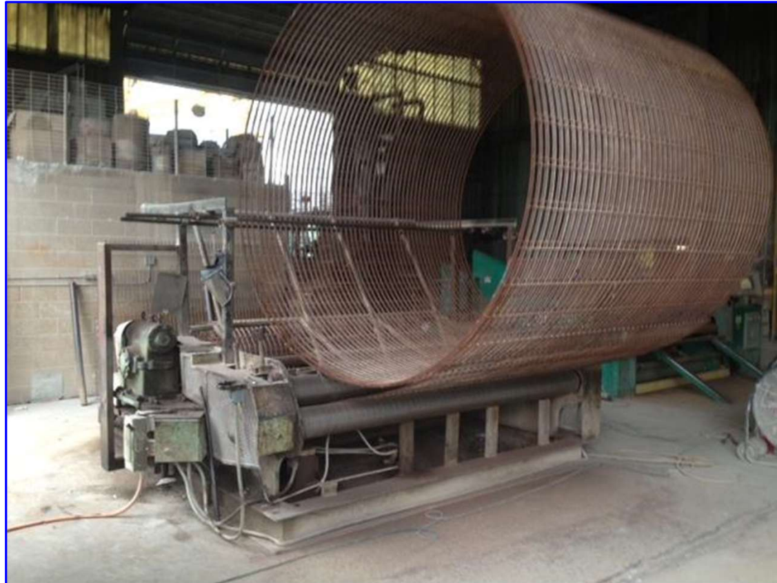
Cage Machine Set Up w/ Safety Bar Through The Cage
