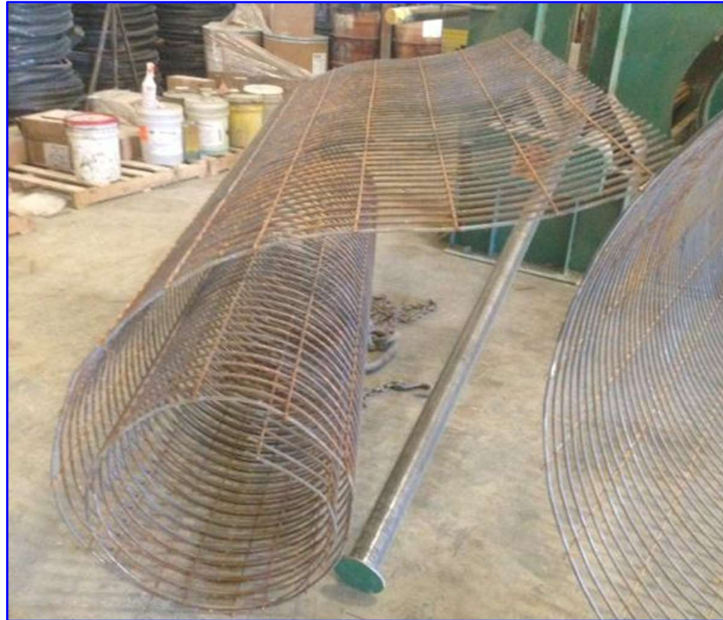
Improper Mesh Rolling Machine Set Up
