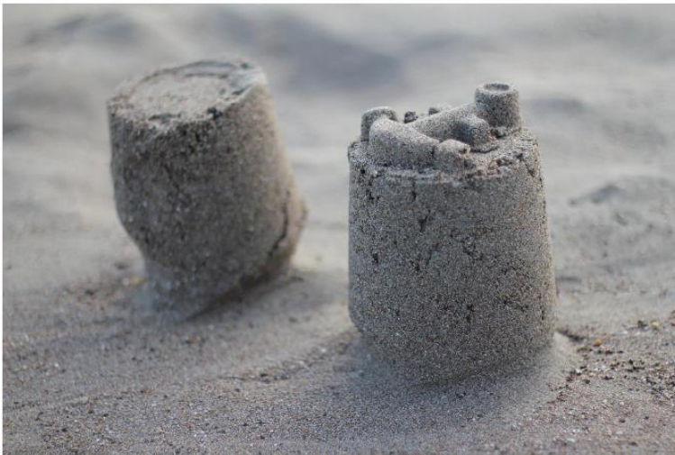
Figure 57. Sandcastles ready to collapse due to saturation by the incoming tide. Excess water fills air voids and results in loss of suction stress between particles and results in slumping (free image Pixabay).
