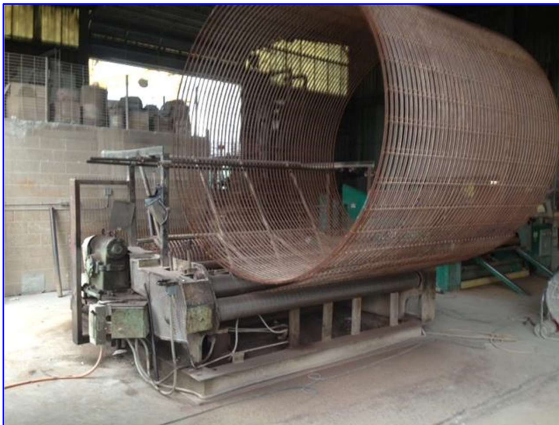
Cage Machine Set Up w/ Safety Bar Through The Cage
