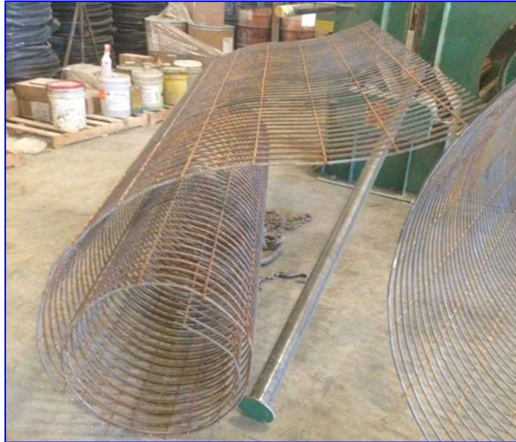
Improper Cage Machine Set Up
