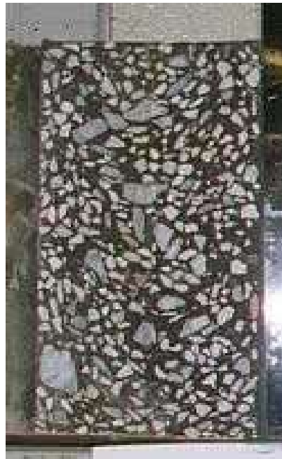
Aggregate at top No Segregation
