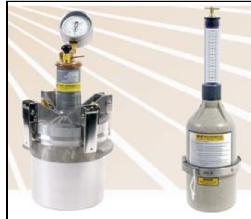
ASTM C173 Air Content of Freshly Mixed Concrete by Volumetric Method
