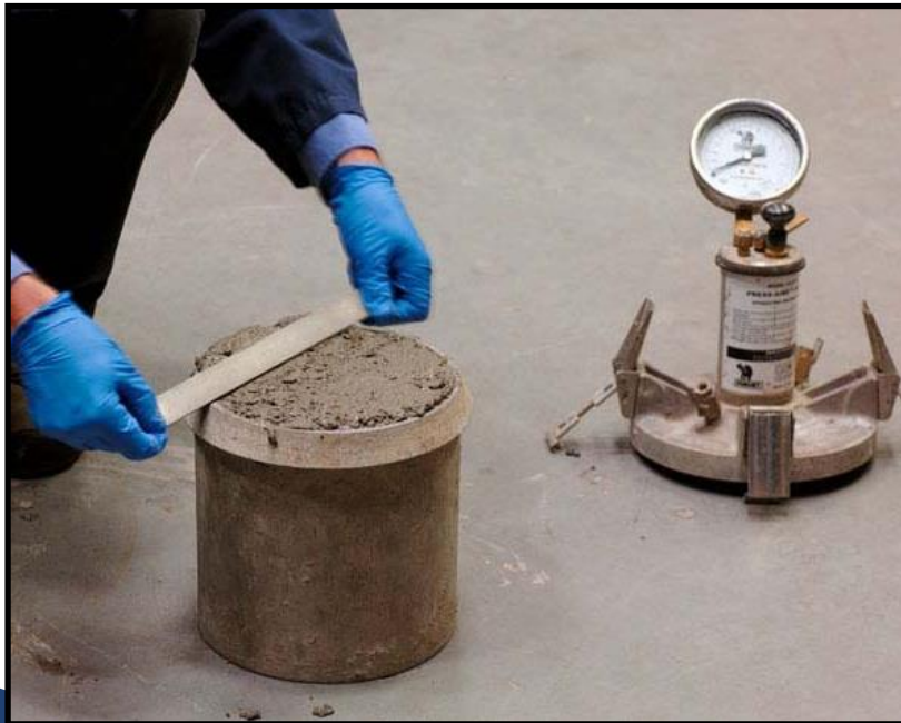
ASTM C231 Test Method for Air Content of Freshly Mixed Concrete by the pressure method
