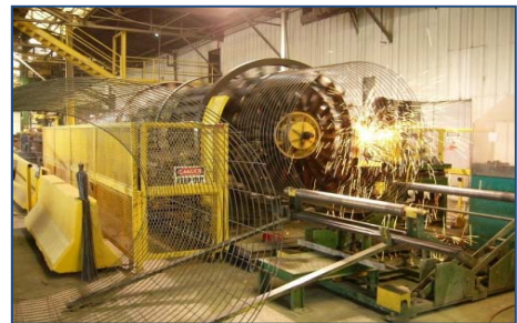
Fig. 1-10. Automatic cage welding machine.
