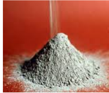
Fig 2-2. Portland cement: a fine powder that when mixed with water becomes the glue that holds aggregates together in concrete.
