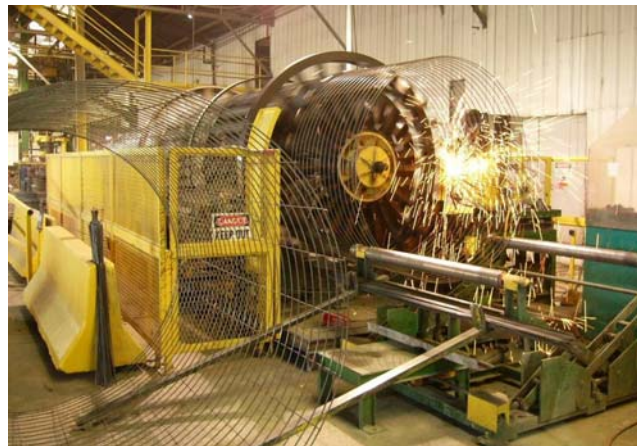
Fig 1-4. Welding machine for reinforcing cages.
