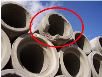
Fig. 2-1. Illustration of damaged pipe.
