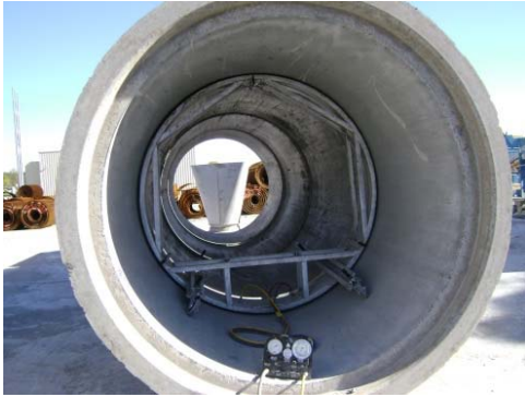
Fig. 3-12. Internal joint test.
