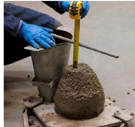
Figure 3-2. Illustration of a slump test.
