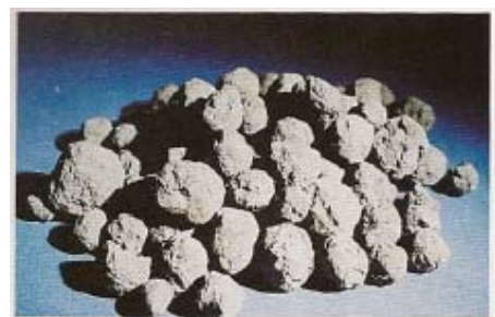
Fig 2-8. Portland cement clinker; about 20 mm in diameter.
