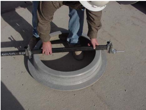
Fig. 2-1. Example of an equipment dimension inspection being taken.
