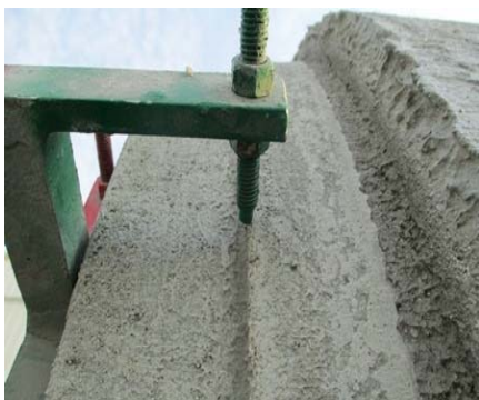
Fig. 1-6. Application of Go/No-Go Gauge to pipe.
