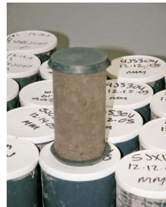
Fig. 3-9. Illustration of core samples removed for concrete for testing.
