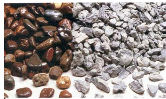
Fig. 4-2. Coarse aggregate; rounded gravel and crushed stone.
