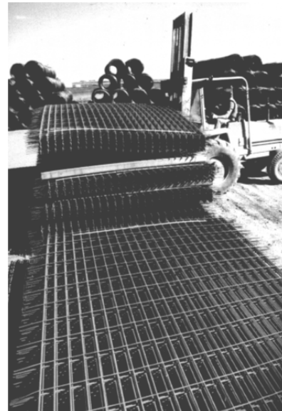
Fig. 6-4. Welded wire reinforcement sheets (courtesy of Wire Reinforcement Institute).
