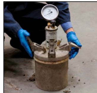
Fig. 3-3. Illustration of pressure testing concrete.
