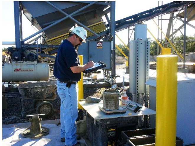
Fig. 3-1. Equipment setup for the ASTM Pressure Meter Air Test for Concrete.
