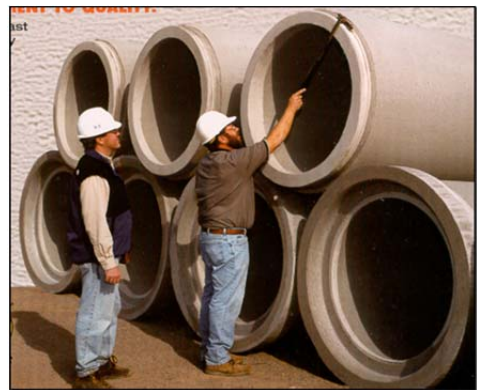
Fig. 1-1. Illustration of visual inspection of finished product.
