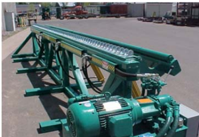
Fig. 1-9. Wire mesh bender used in fabrication of box culvert reinforcing.
