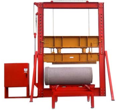
Fig. 3-1. Three-edge bearing testing equipment.
