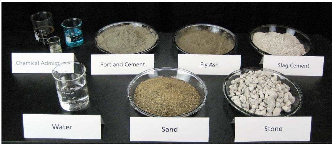
Fig 1-1. Components of concrete mix design.
