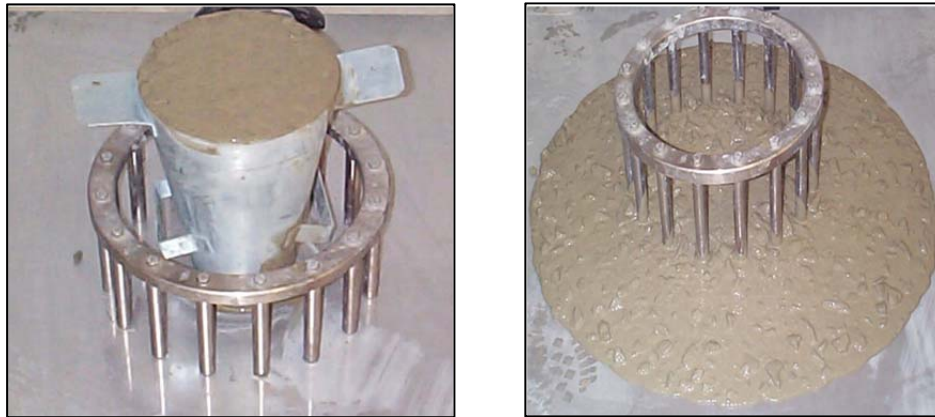
Fig. 3-7. Illustration of rapid assessment test being performed for self consolidating concrete.
