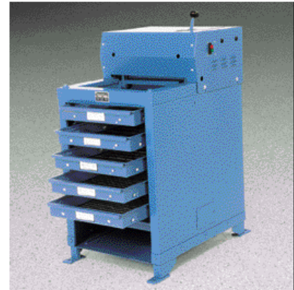
Fig. 4-13. Aggregate Screen Shaker.
