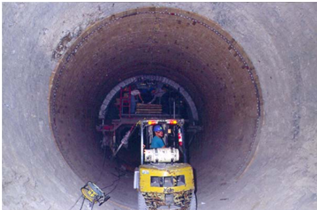
Fig. 2-7. Inside the Kiln: Diameters can range from 12 to 24 ft.
