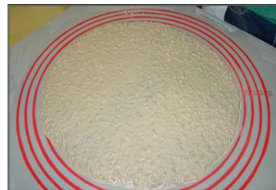
Fig. 7-3. SCC slump flow evaluation.
