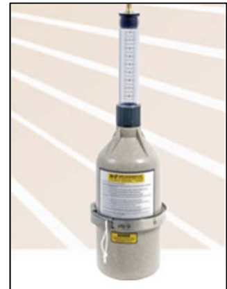
Fig. 3-4. Illustration of volumetric air meter for fresh concrete.
