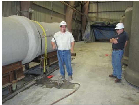
Fig. 3-13. External joint test.
