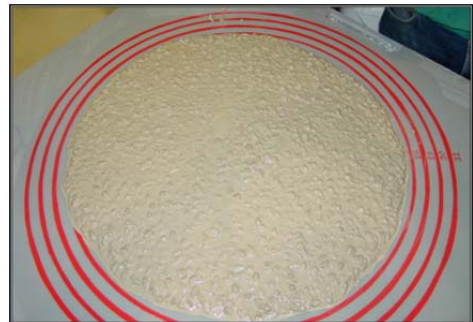
Fig. 1-13. SCC slump flow evaluation.
