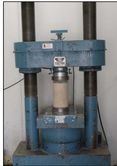
Fig. 3-8. Illustration of concrete compression testing equipment.
