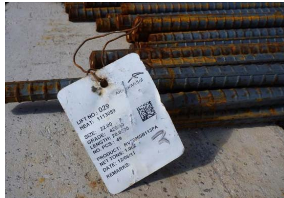
Fig. 6-2 Photo of rebar with identification tag.
