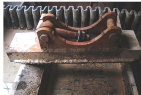
Fig. 3-9. Example of vibrator mounting bracket welded to the form stiffeners.
