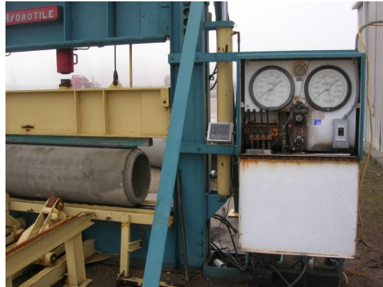
Fig 3-2. Illustration of a three-edge bearing test.
