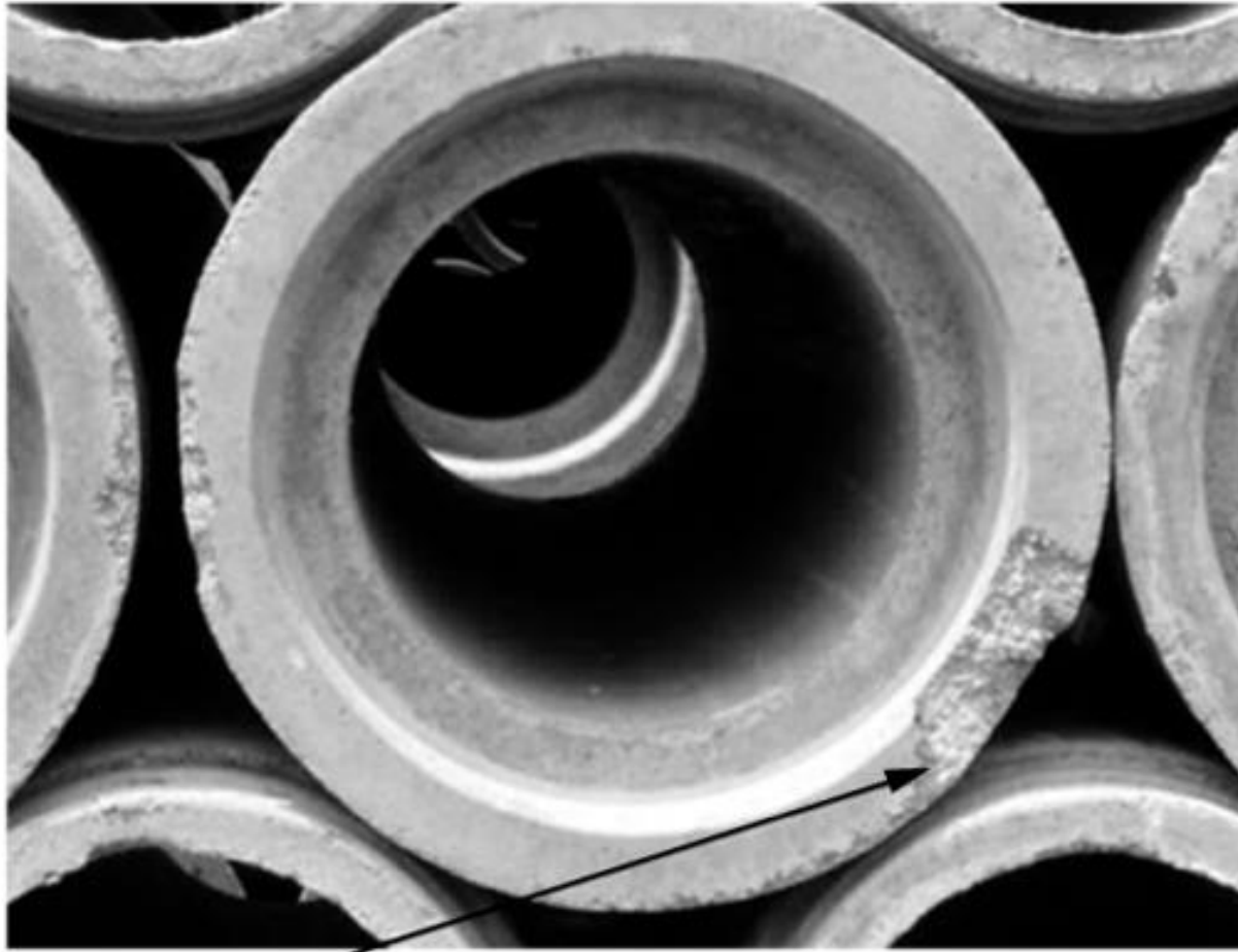
Figure 18 —Repairable Chip on Bell End (Photo Courtesy of ACPA)
