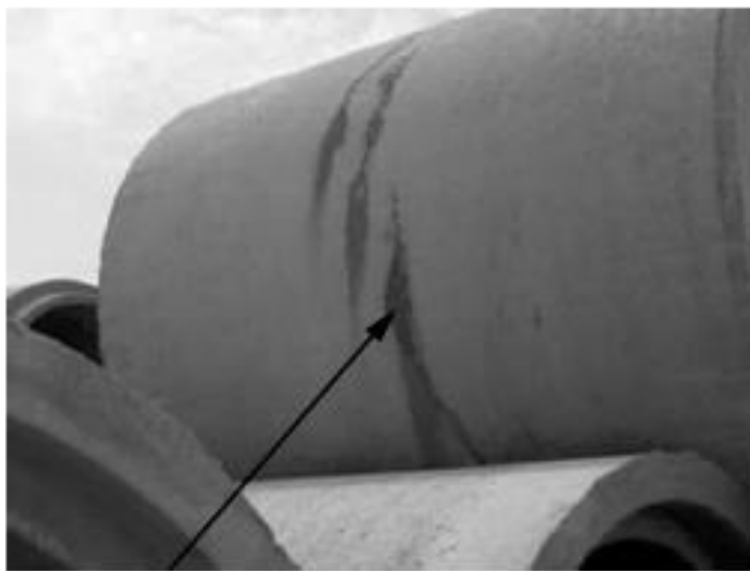
Figure 27—Rejectable Pipes with Cracks Passing through the Wall and Exceeding 0.01 in. in Width and 12 in. in Length (Photos Courtesy of ACPA)
